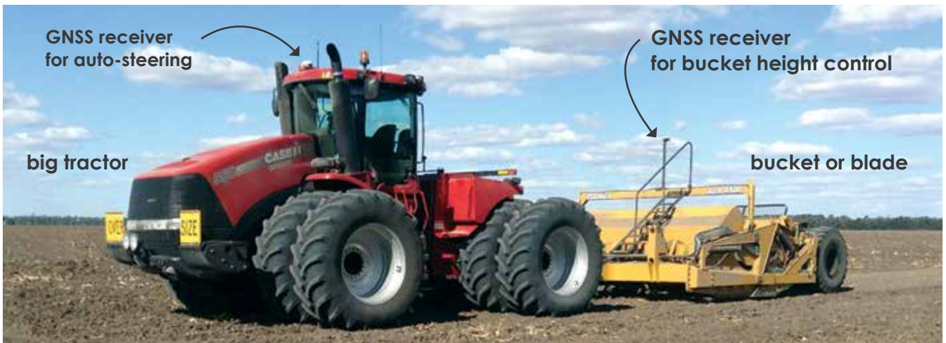
The components of a GNSS levelling system.
